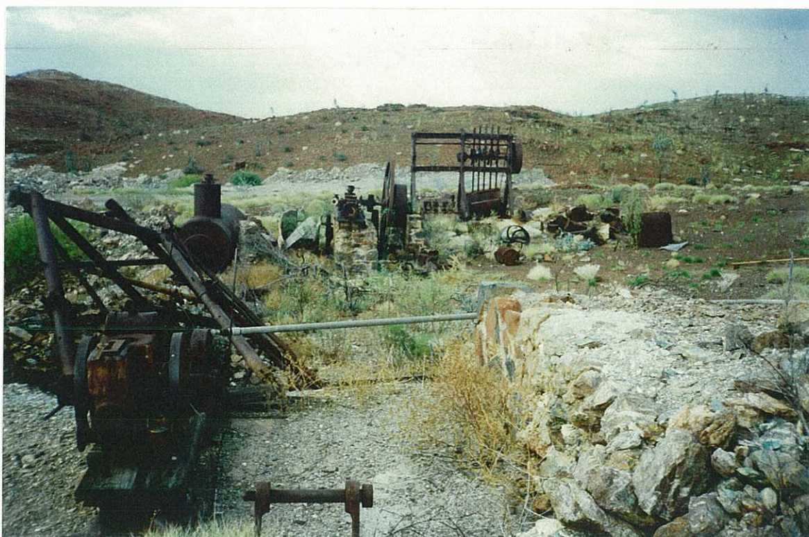
The remnants of the 10 stamp battery and other mining equipment.
