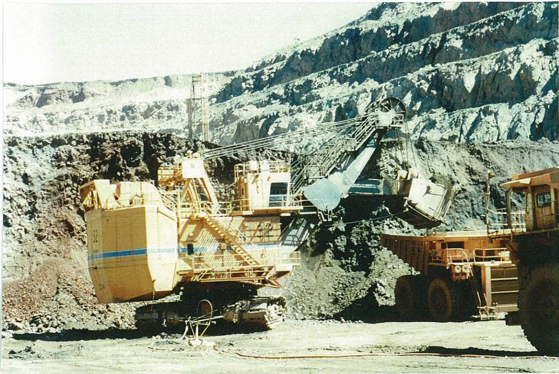
An electrical shovel at work in the pit. loading ore onto a Liebherr 240R truck. This shovel picks up about 70 tonnes at one go and is powered by 11,000 volts of electricity (see cable in foreground).
