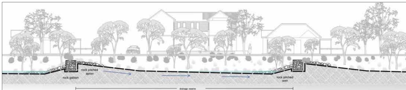
Figure 33: Typical section through drainage corridor
