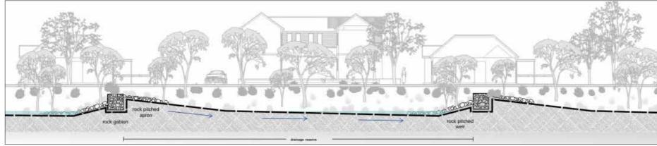
Figure 33: Typical section through drainage corridor
