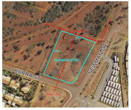
Whilst significantly larger than the minimum 2,500m<sup>2</sup> sought for the facility, the additional size allows for the development to accommodate the high voltage power line that runs through the site.
