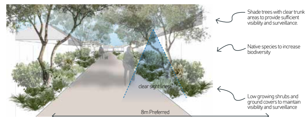
P2 - Figure 27: Typical section Pedestrian Access Ways
